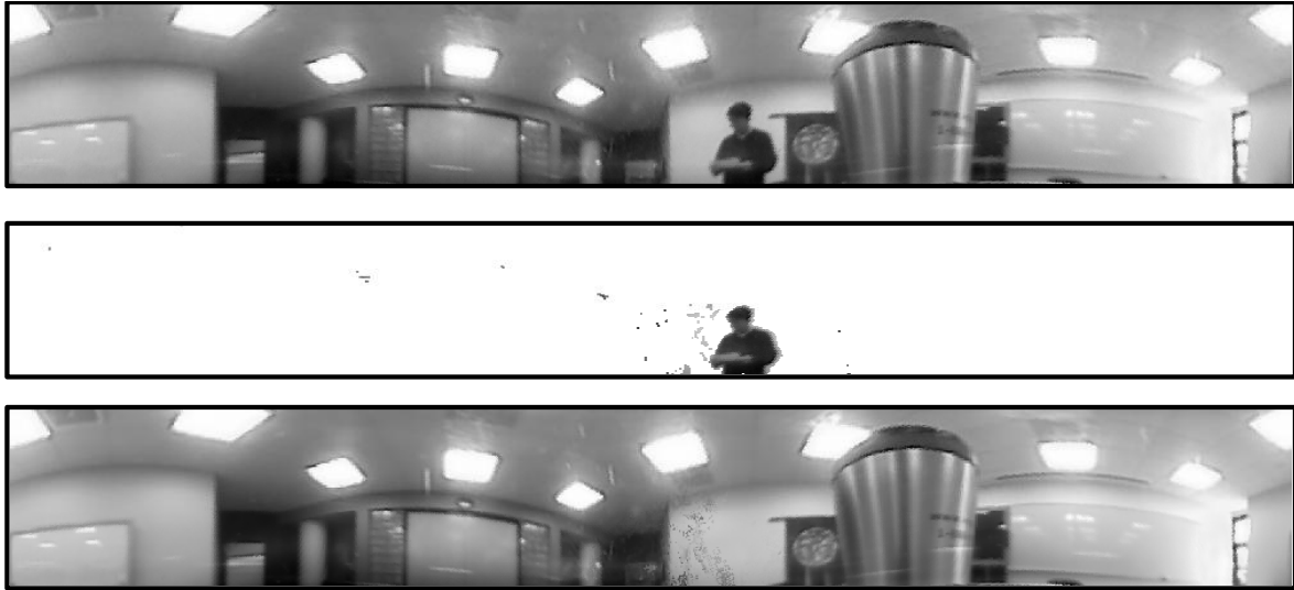
Figure 6. From top to bottom, examples of a panoramic video frame, the extracted foreground and the background image.
